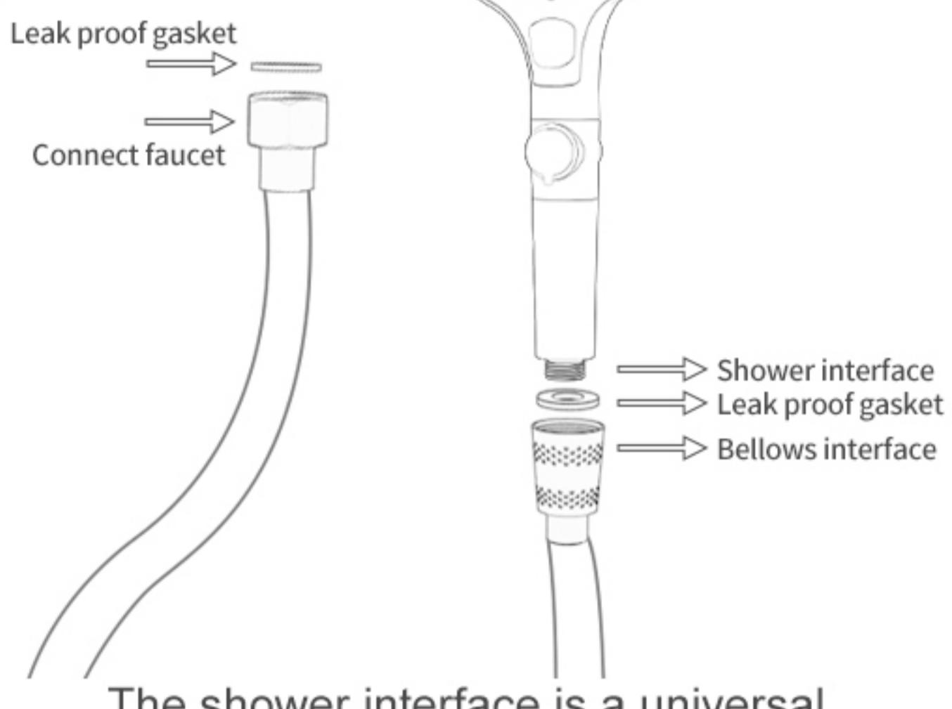
The shower interface is a universal interface that can be directly tightened clockwise with the shower pipe.
