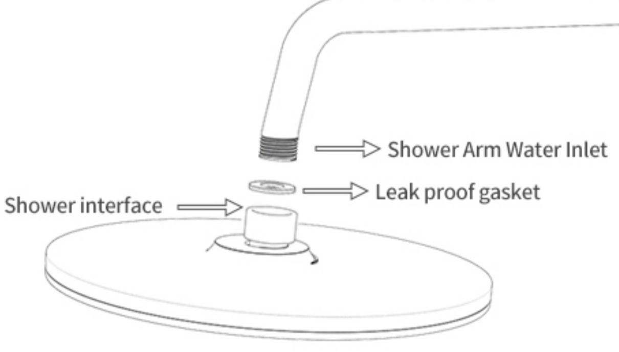
The interface of the showerhead is a G1/2 universal interface. After receiving it, ensure that there is a gasket inside the interface and simply screw it on to use it
