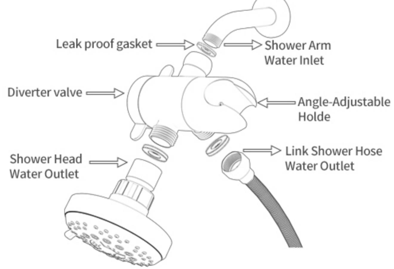
Note: Before installation, please ensure that there is a washer inside the nut, otherwise there may be water leakage
