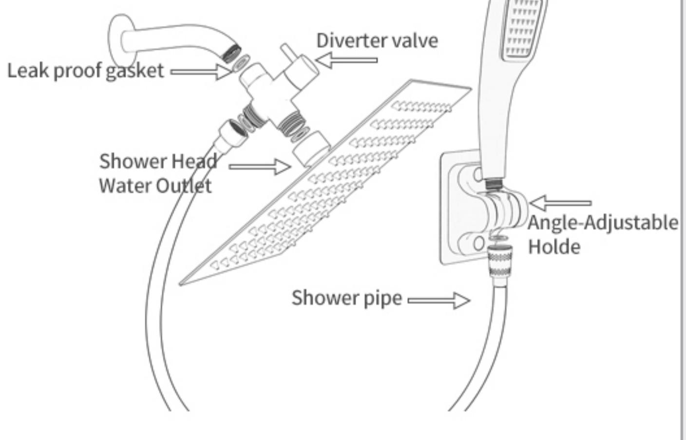
Note: Before installation, please ensure that there is a washer inside the nut, otherwise there may be water leakage
