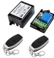
QIACHIP DC 12V 1CH 433Mhz RF Wireless Relay Remote Control Light Momentary... 591 $12 99
