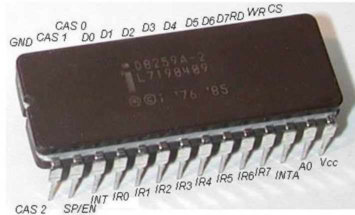
8259A PIC Microcontroller with all pins labeled.
